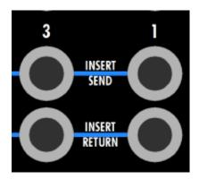
$\underline{\text{INSERT SEND}}\colon$  ¼" tip-ring-sleeve, balanced, low-impedance, line-level
