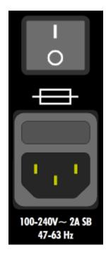
POWER SWITCH: On/off AC power switch
