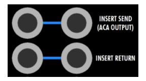
INSERT SEND (ACA OUTPUT) (LEFT & RIGHT): 1/4" tip-ring-sleeve, balanced, low-impedance, line-level
