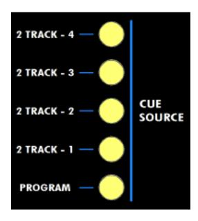
In addition the stereo cue bus, the C/R SOURCE selections (PROGRAM\*) and up to four (4) external stereo sources can be routed to the cue master. These additional cue sources are selected using the CUE SOURCE selector switches and routed to the cue master via CUE SOURCE level control.
