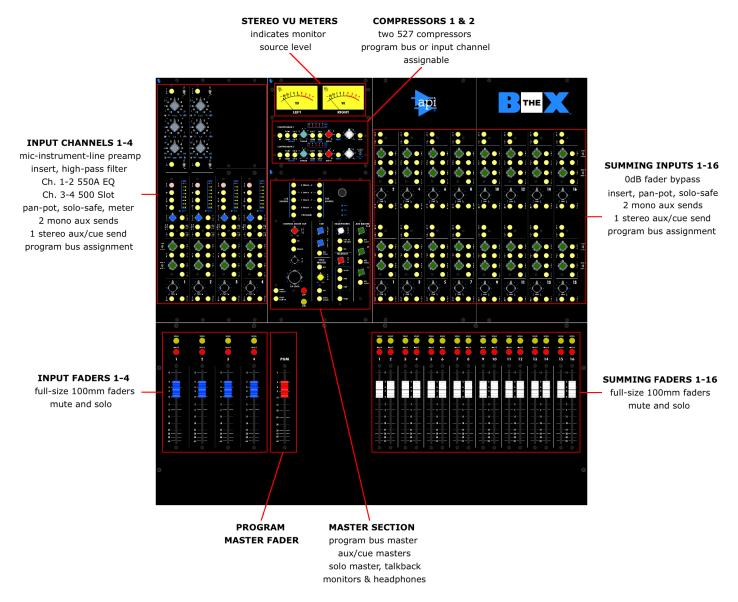
For recording, "The BOX" provides four (4) input channels. Channels 1 & 2 are equipped with preamp, filter, built-in 550A equalizer, insert, assignable compression, and output routing. Channels 3 & 4 provide the same features, but are each equipped with an API 500 series slot instead of the built-in EQ.
