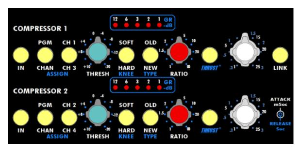
To use the compressors while mixing, they need to be assigned to the program bus, with Compressor 1 assigned to Left side of the program bus and Compressor 2 assigned to the Right. The compressors are located after the PROGRAM SUM INPUT and pre-insert.
