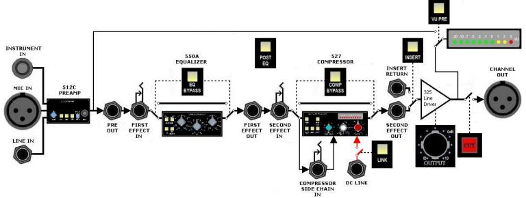
NOTE: The order of the First and Second Effect jacks on the rear panel does not change with the compressor when the POST EQ switch is engaged.
