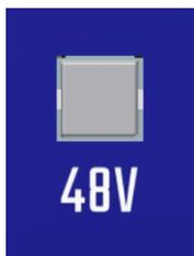
**48V:** Engage to apply 48-volt phantom power to the microphone INPUT
