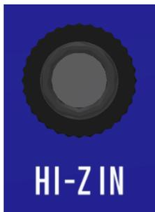
**HI-Z IN:** High-impedance, 500k $\Omega$ , unbalanced instrument input
