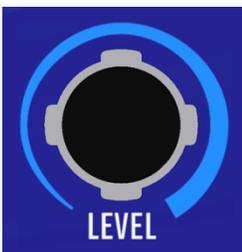
**LEVEL:** Trims (attenuates) the level of the output stage
