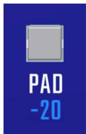
**PAD -20:** Toggle to apply 20dB of attenuation to the input signal
