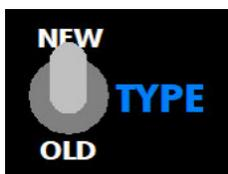
**TYPE**: Toggle to select the compressor circuit topology
