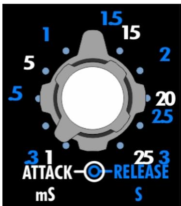
Attack and Release times are controlled via a dual-concentric potentiometer. The outside pot (ring) controls attack time and the inside pot (center) controls release time. For ease of understanding these controls are show separately below.
