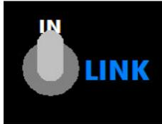
**LINK**: Set to engage DC control voltage summing with other units
