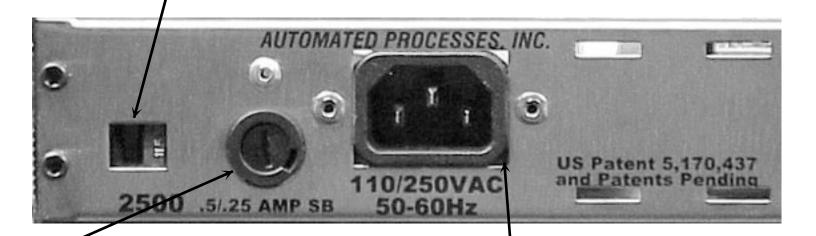
FUSE HOLDER REPLACE WITH A TYPE 0.5A slow-blow for 90-125 VAC 0.25A slow-blow for 200-250 VAC AC INLET CHECK VOLTAGE SELECTOR BEFORE TURNING 2500 ON
