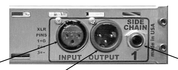
XLR INPUT +4dBu Pin 2 HOT XLR OUTPUT +4 dBu Pin 2 HOT SIDE CHAIN INPUT , +4dBu Normals to XLR INPUT
