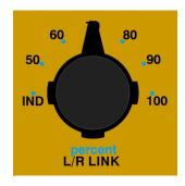
**L/R LINK**: Sets the percentage of the control voltage link between the Left and Right channels
