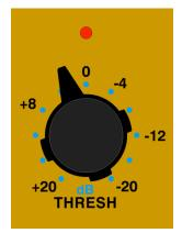
**THRESHOLD**: Sets the level at which compression begins
