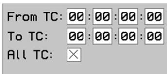
**Timecode Range:** Selects the range of timecode to which the Offline Trim function will be applied. Either all timecode addresses or a range of addresses with user-defined beginning and ending points can be selected.
