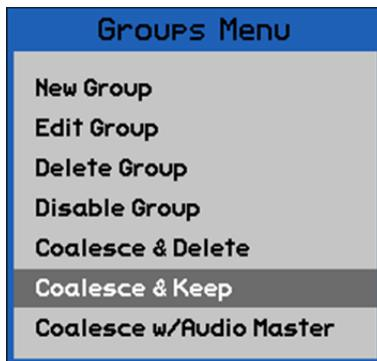
Selecting "Coalesce & Keep Group" will cause the automation system to create a new mix in the Mix Tree with the following attributes:
