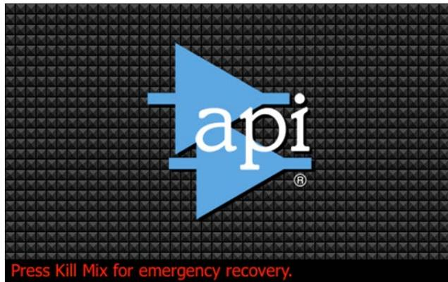
5. Press the KILL MIX button while this screen is being displayed to initiate the emergency recovery procedure. You will only have a few seconds. The emergency recovery will begin.
