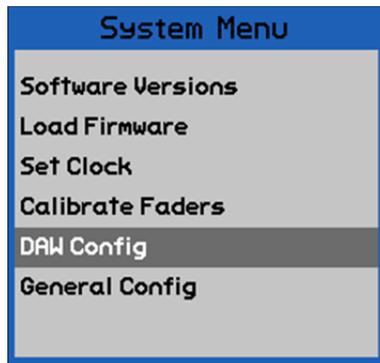
To use DAW control, the system must be first configured. This involves mapping the four pairs of MIDI ports with the 8-channel Fader Modules. This is accomplished using the "DAW Config" dialog box, available from the System Menu.
