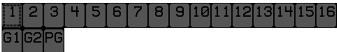
The numbered channels are associated with the input channels. G1 and G2 are the two Control Group Master Faders and PG is the Program Master Fader.
