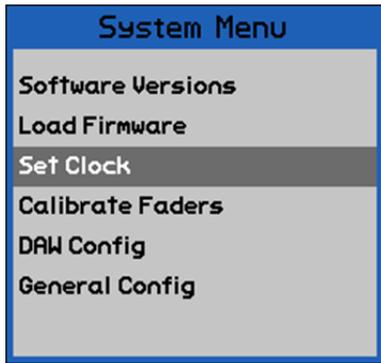
To set the system clock, highlight "Set Clock" in the System Menu and press the SEL (Select) button.
