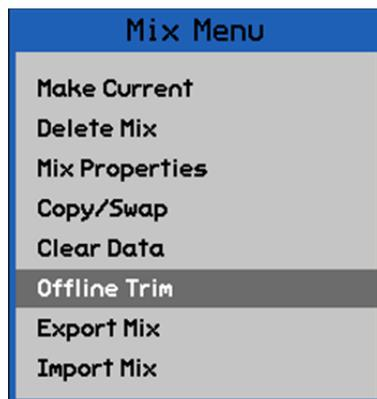
The "Offline Trim" menu item facilitates fader data trimming within the highlighted mix.
