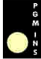
The Program Insert (PGM INS) switch on the 268B program master module can be used as the "Insert Group Master" when that Program Master fader is designated as a "Group Master Fader." However, insert groups can be set up independently of fader groups.
