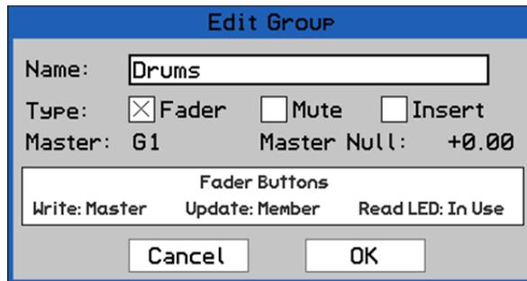
To change the name of the selected group, highlight the "Name:" text-entry field and press the SEL (Select) button. Using the text-entry procedures, edit the existing name or enter a new one. Press ESC (Escape) once the name has been edited.
