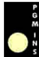
The PGM INS (Insert) switch on the 268B Program Master Module is typically used as the "Insert Group
