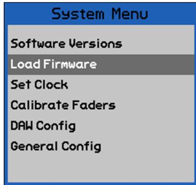
Highlight "Load Firmware" in the System Menu and press the SEL (Select) button.
