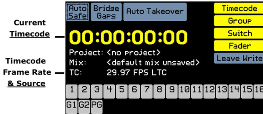
The current timecode address, frame rate, and source are displayed on the Status Page.
