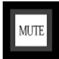
The MUTE switch on the 548B Input Module is typically used as the "Mute Group Master" when that channel is designated as a "Group Master Fader." However, mute groups can be set up independently of fader groups.
