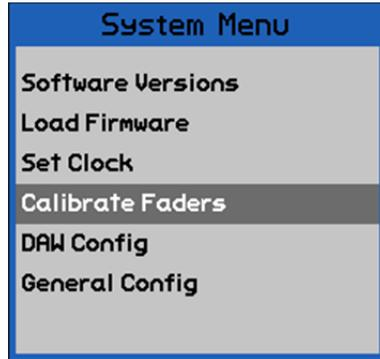
To calibrate faders, highlight "Calibrate Faders" in the System Menu and press the SEL (Select) button.
