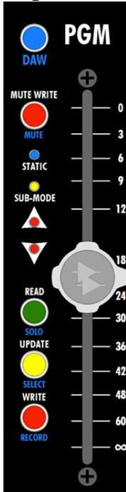
The Program Master fader on the Automation Controller can also be designated as a Group Master for faders and inserts.
