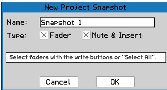
The New Project Snapshot dialog box allows a new snapshot to be named.
