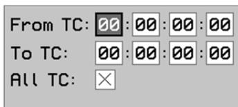
To select the "From" and "To" timecode addresses, highlight the needed field and press the SEL (Select) button. The field will turn grey. Use the Jog-Wheel to select the needed value and press the SEL (Select) button.
