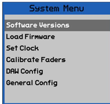
To view the currently loaded software versions, highlight "Software Versions" in the System Menu and press the SEL (Select) button.
