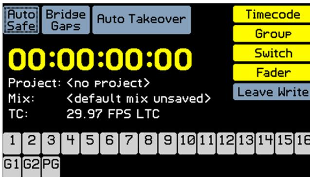
Once the firmware is loaded the default Status page will be displayed and the system is ready to create a new Project file or load and existing one.
