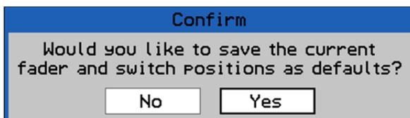
Highlight "Yes" button and press the SEL (Select) button to save the current fader, mute, and insert positions as the Default Positions.
