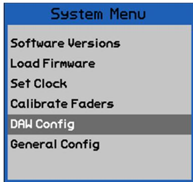
To use DAW control, the system must first be configured. This involves mapping the four pairs of MIDI ports with the 8-channel Fader Modules. This is accomplished using the "DAW Config" dialog box, available from the Main Menu.
