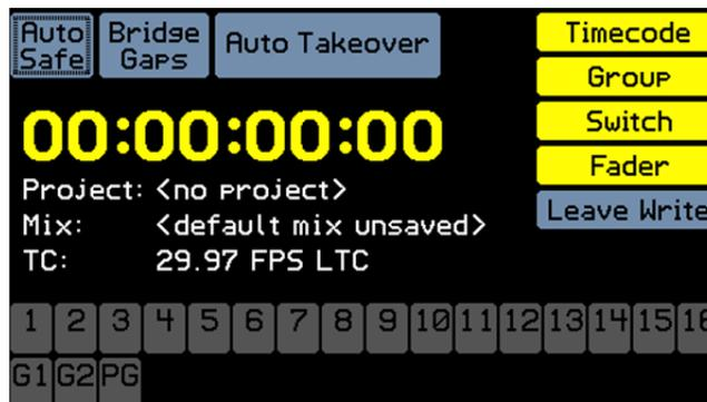
The channel grid displays the current mode of each channel and its selection status. It also provides the means for mode assignment.
