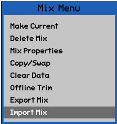
The "Import Mix" menu item facilitates the importing of .VMX mix files into the currently open project and Mix Tree.
