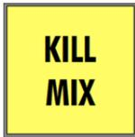
KILL MIX: Suppresses end-of-pass processes when timecode is stopped. It activates a flag to discard any changes made during the current automation pass.
