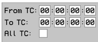
**Timecode Range:** Selects the range of timecode to which the Copy/Swap function will be applied. Either all timecode addresses or a range of addresses with user-defined beginning and ending points can be selected.
