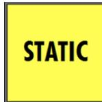
Press the STATIC button to engage the STATIC sub-mode on all channels. This will allow WRITE mode to be engaged from the Automation Controller (ACM) without being in UPDATE first.
