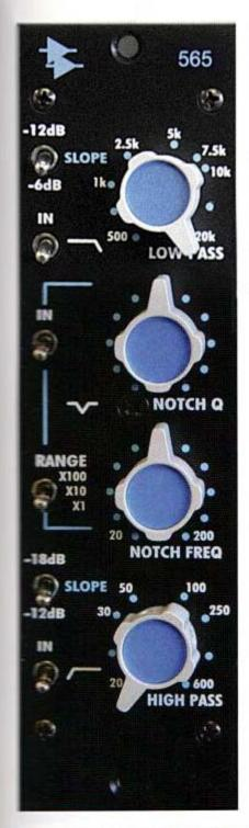
The unit starts at the top with a 500 Hz to 20 kHz Low Pass Filter with a switchable slope of 6 or 12 dB/octave. Skipping over the Notch filter for a moment, the High Pass Filter at the bottom of the module has a range of 20 Hz to 600 Hz with a choice of 12 or 18 dB/octave slopes.
