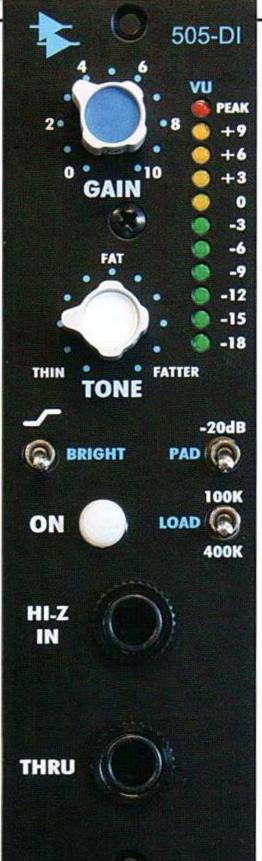
Next to this is an 8 kHz Bright Boost that adds about 10 dB of high end. It works especially well on acoustic guitars, giving them a much-needed sparkle and string definition when recording direct. I like this definition on DI bass too, for when I want to hear the string plucks. Taken in tandem, the Tone control, impedance switching, and Bright Boost offer a simple but effective way to get your incoming signal sounding full and clear prior to adding EQ and further processing.
